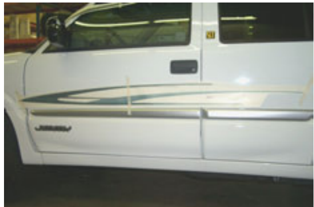
2. Tape the component graphic panels onto the side of vehicle to determine exactly where you want the graphic panels installed. Apply a strip of tape vertically through the center of each component and lightly tape each end of the graphic panel to the vehicle.
