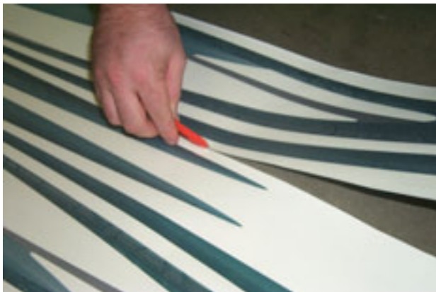
1. Using your Snappy knife, carefully cut the component graphics apart from each sheet, if needed.
